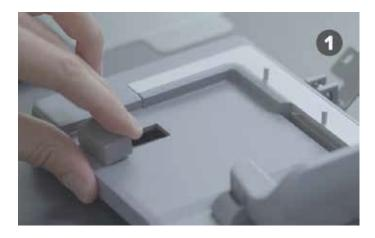
Insert the smartphone without the case and release the upper clip
