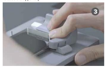
Push the lower clip to lock and fix the smartphone in position
