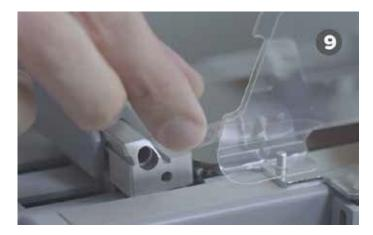
Insert the glass in the appropriate guide-pins
