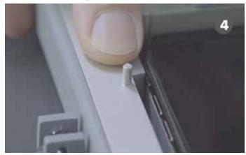
If the spacer of the smartphone is greater than the edges, lower the metal lever
